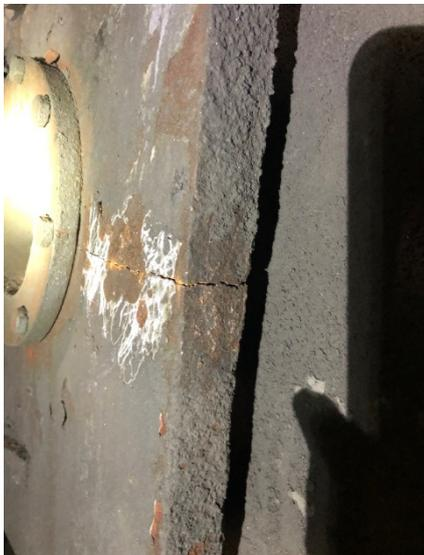
Figure 3. Initial crack on filter press pressure end
