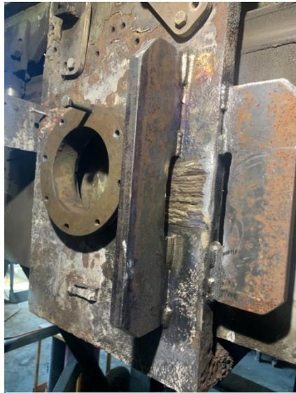
Figure 4. Area completed with "strong backs" installed
