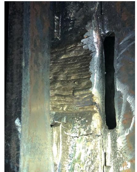
Figure 5. New crack after repair just below the repair job
