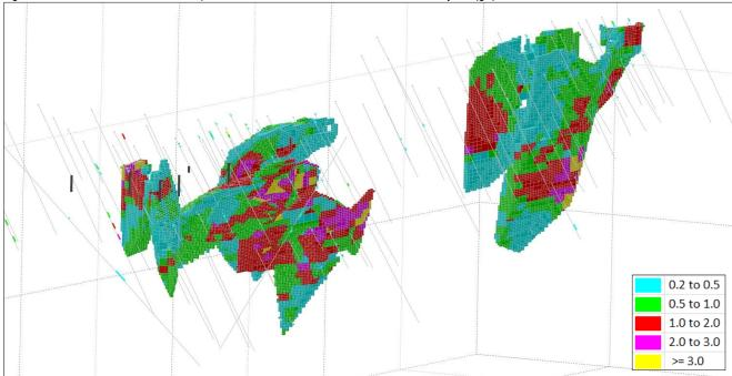
Figure 22: Melbourne Bitter 3D view looking down to the north-west showing drill holes, historic shafts, and OK block model coloured by Au (g/t)
