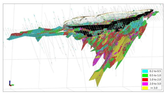
Figure 18: Kingfisher 3D view looking down to the north-west showing drill holes and OK block model coloured by Au (g/t)
