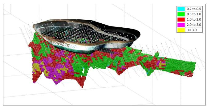
Figure 24: Hawk 3D looking down to the north-east showing drill holes and OK block model coloured by Au (g/t)
