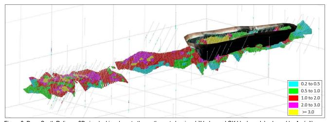
Figure 8: Deep South Reliance 3D view looking down to the north-west showing drill holes and OK block model coloured by Au (g/t)
