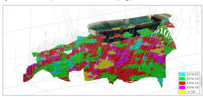
Figure 28: Heron South 3D looking down to the north-west showing drill holes and OK block model coloured by Au (g/t)
