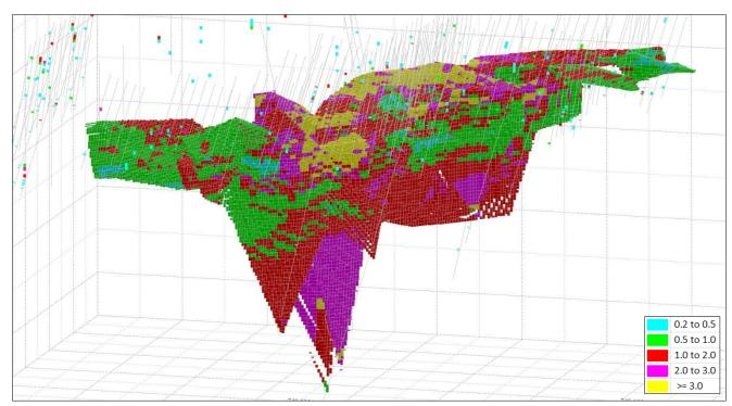
Figure 26: Heron 3D looking down to the east-southeast showing drill holes and OK block model coloured by Au (g/t)
