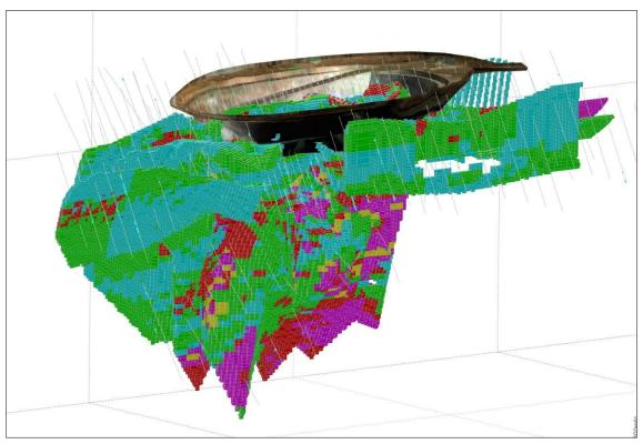
Figure 10: Eagle 3D view looking down to the north-west showing drill holes and OK block model coloured by Au (g/t)
