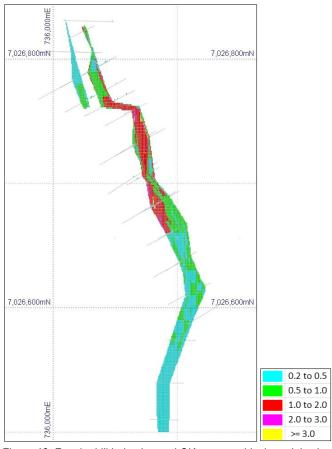
Figure 13: Fangio drill hole plan and OK resource block model coloured by Au (g/t)
