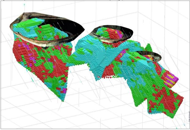
Figure 16: Kearrys 3D view looking down to the north-east showing drill holes and OK block model coloured by Au (g/t)
