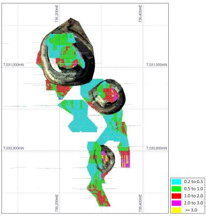
Figure 15: Kearrys drill hole plan and OK resource block model coloured by Au (g/t)
