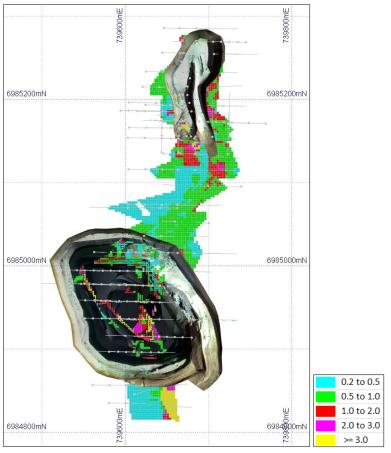
Figure 31: Wedge drill hole plan and OK resource block model coloured by Au (g/t)
