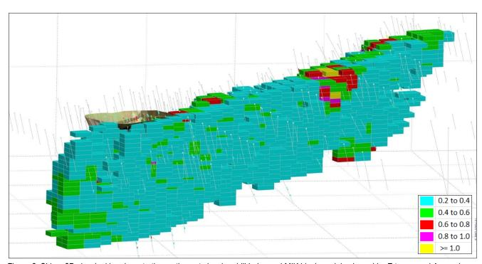
Figure 6: Shiraz 3D view looking down to the north-west showing drill holes and MIK block model coloured by E type panel Au grade (g/t).
