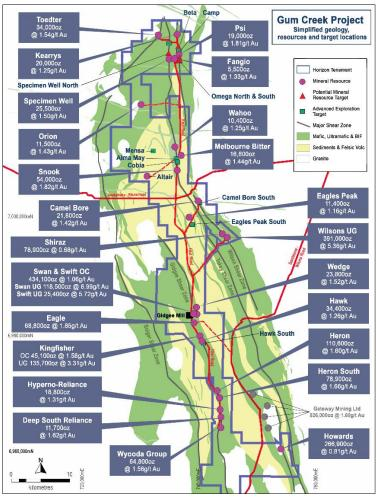
Figure 2: Gum Creek Gold Project Mineral Resources, Advanced Mineral Resource Targets and Exploration Targets over simplified geology<sup>3</sup>
