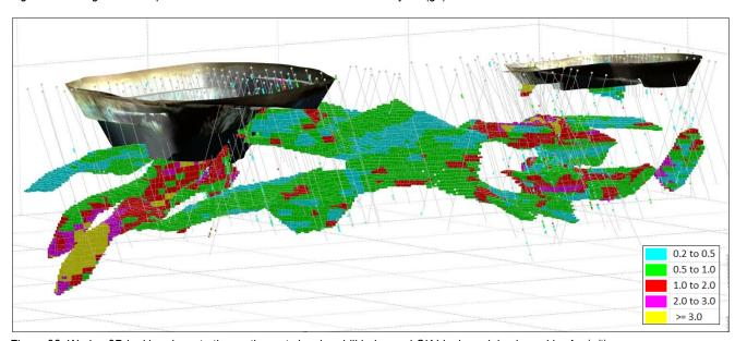
Figure 32: Wedge 3D looking down to the north-west showing drill holes and OK block model coloured by Au (g/t)
