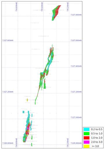
Figure 29: Specimen Well drill hole plan and OK resource block model coloured by Au (g/t)
