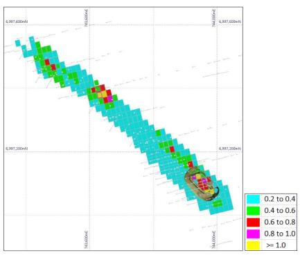
Figure 5: Shiraz drill hole plan and MIK resource block model coloured by E type panel Au grade (g/t).
