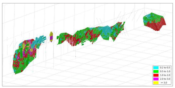
Figure 30: Specimen Well 3D looking down to the north-west showing drill holes and OK block model coloured by Au (g/t)
