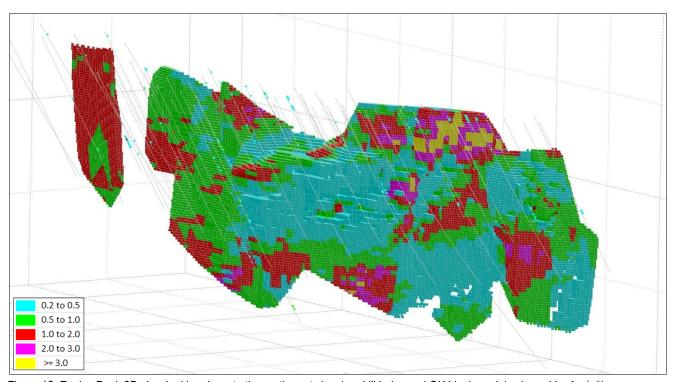
Figure 12: Eagles Peak 3D view looking down to the north-east showing drill holes and OK block model coloured by Au (g/t)
