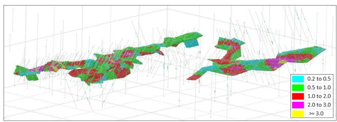
Figure 20: Hyperno-Reliance 3D view looking down to the north-west showing drill holes and OK block model coloured by Au (g/t)
