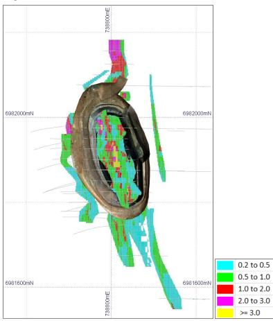
Figure 9: Eagle drill hole plan and OK resource block model coloured by Au (g/t)
