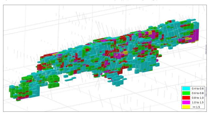
Figure 4: Howards 3D view looking down to the north-west showing drill holes and MIK block model coloured by E type panel Au grade (g/t)
