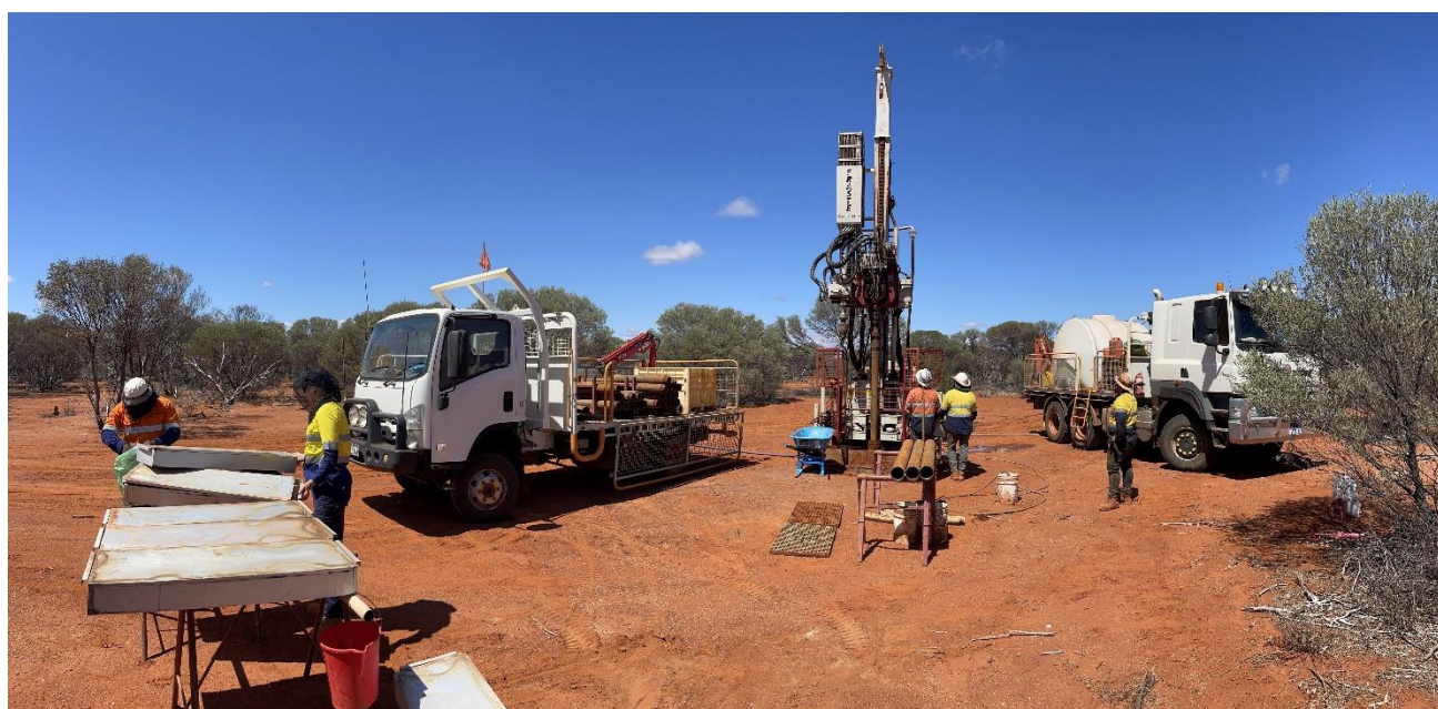
Figure 1: Sonic drilling underway at NiWest Project.
