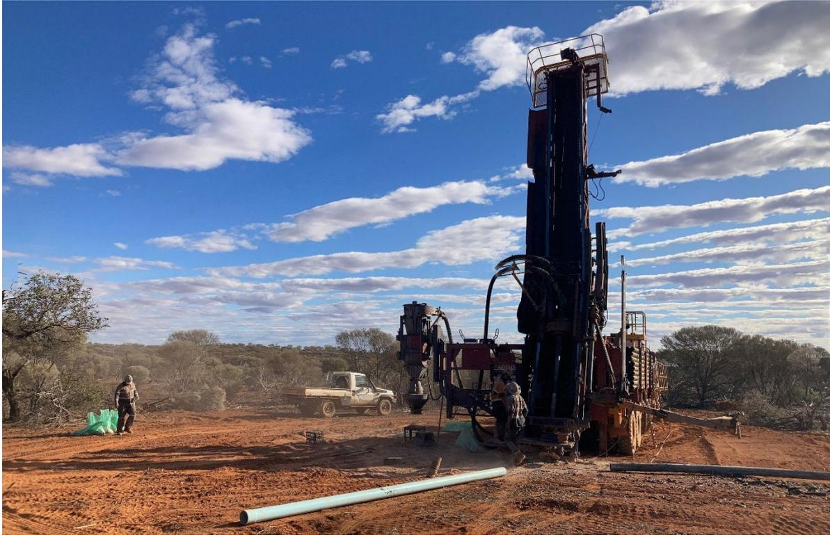
Figure 2: RC drilling at the Mensa Prospect.
