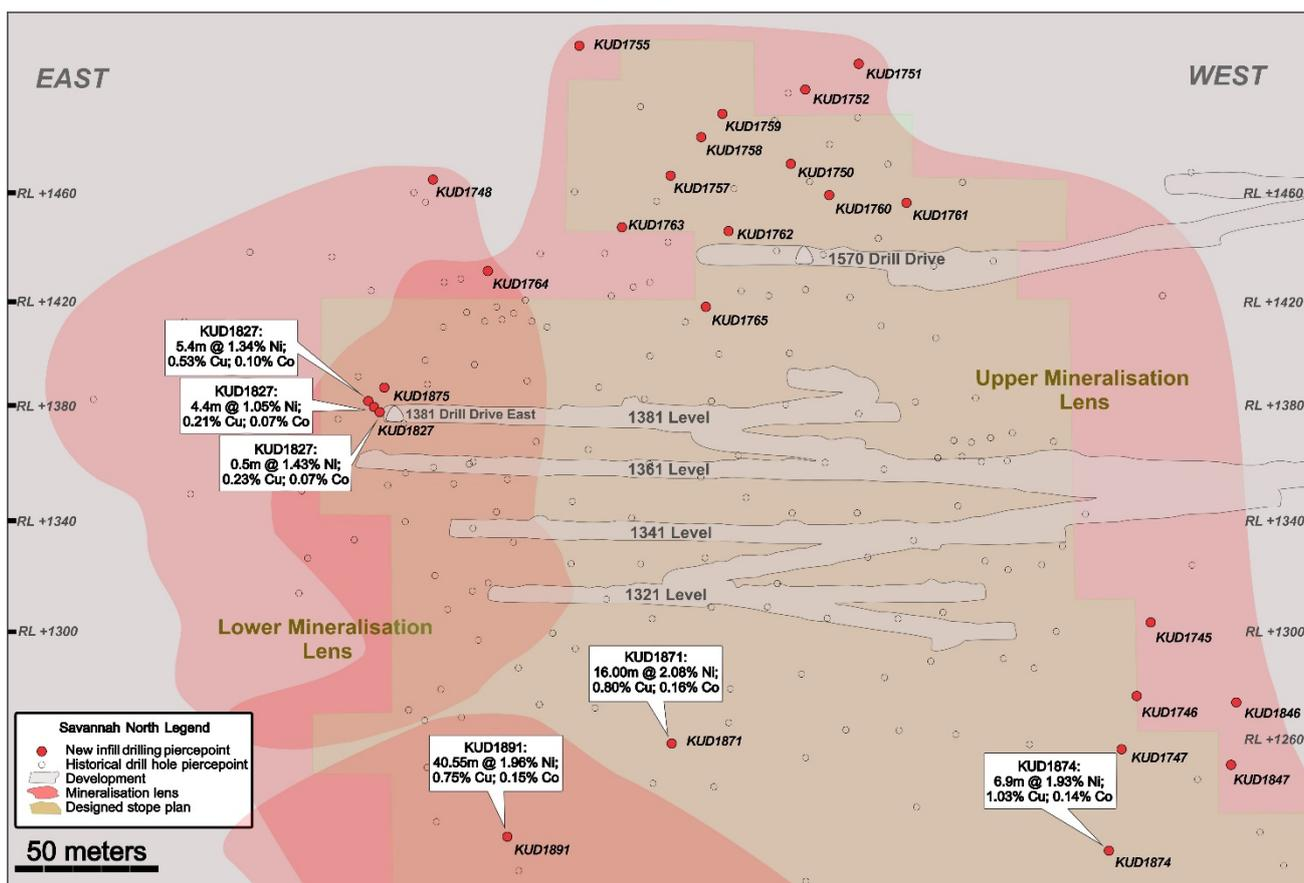
Figure 1: Long-section of the Resource definition drilling at Savannah North and historic Resource definition drilling intercepts with development drives, proposed stope and mineralisation shapes
