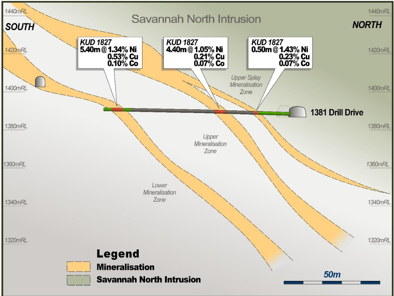
Figure 3: Cross section 6210mE showing drillhole KUD1827 and the three intersections through the multiple splays of the eastern margin of Savannah North
