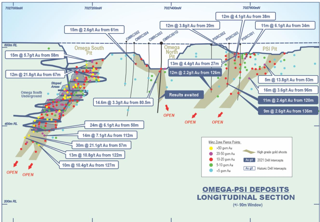
Figure 2: Omega-PSI prospects long section<sup>1</sup> showing gold intercept pierce points coloured by gram x metre (i.e. average intercept grade (g/t Au) multiplied by intercept width in metres), historic open pits, underground infrastructure, interpreted high-grade ore shoots (gold), and 2021 RC intercepts >20 gram x metres labelled (blue).
