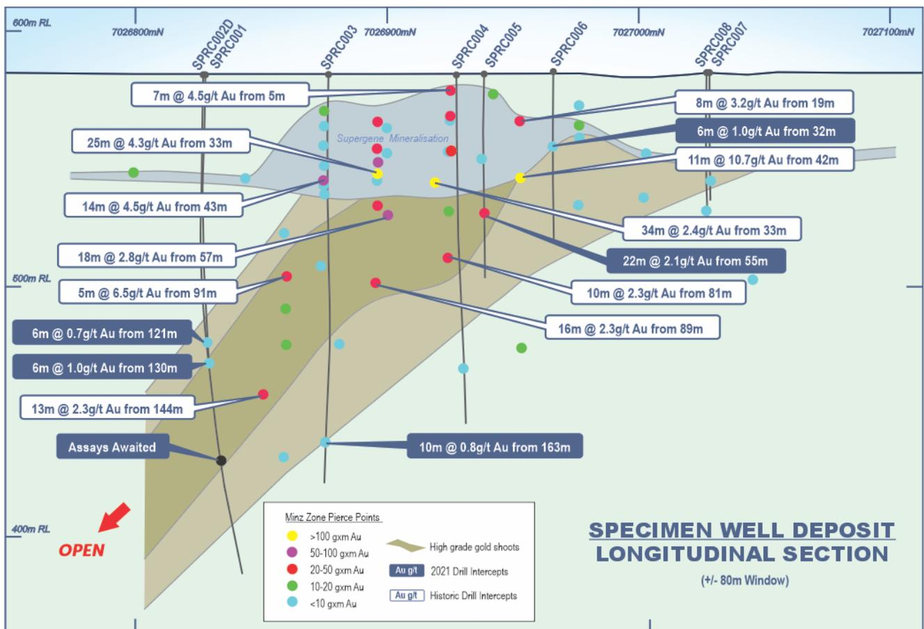
Figure 4: Specimen Well Prospect long section<sup>3</sup> showing mineralised envelopes, and 2021 RC drill intercepts >4 Gxm labelled (blue).
