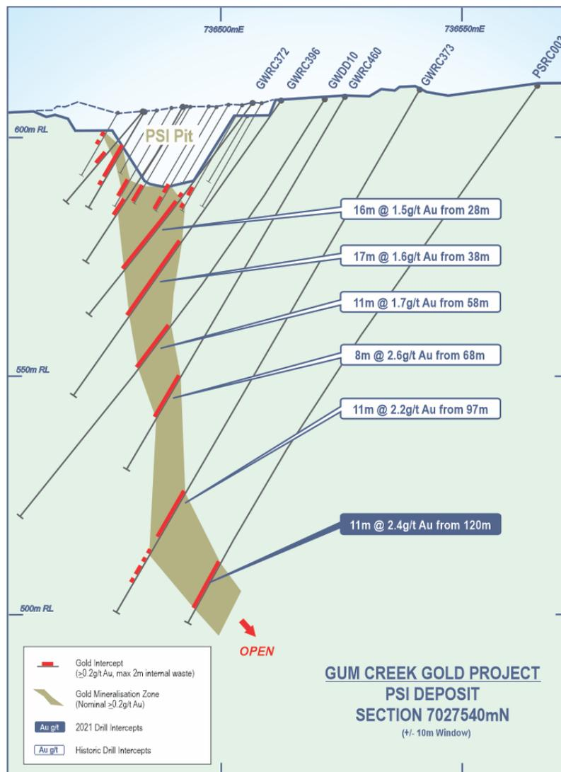
Figure 3: PSI Prospect cross section showing mineralised envelope, >18 GxM previous intercepts<sup>2</sup>, and 2021 RC drill intercept (labelled blue).
