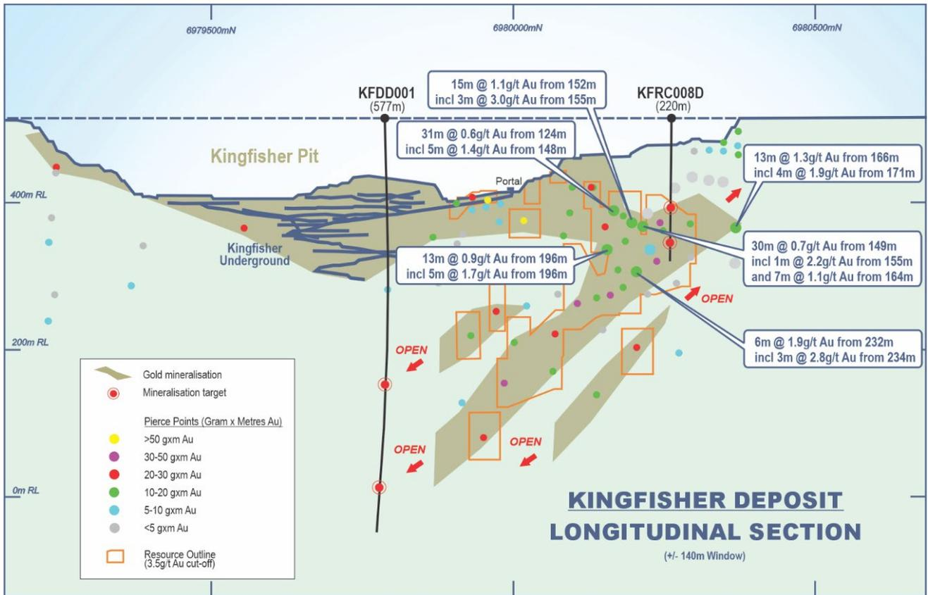
Figure 6: Kingfisher Prospect long section showing gold intercept gram x metre pierce points with recent >10 gram x metre intercepts labelled, current resource outline, open pit, and interpreted high-grade ore shoots.
