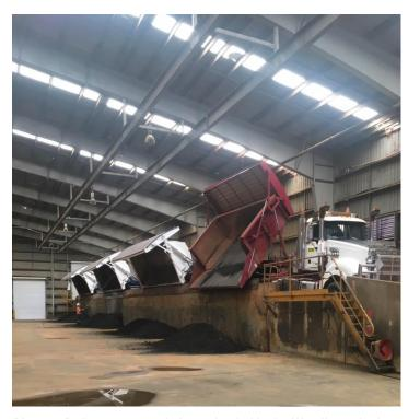
Photo 3: Bulk concentrate being unloaded in the Wyndham shed
