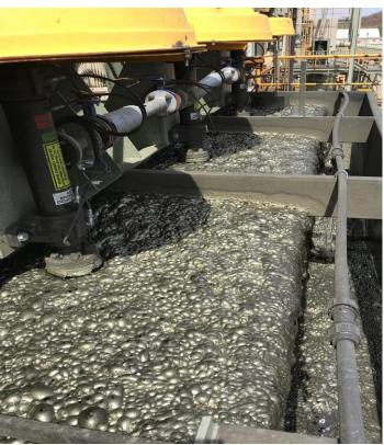
Photo 2: Flotation cells in operation
